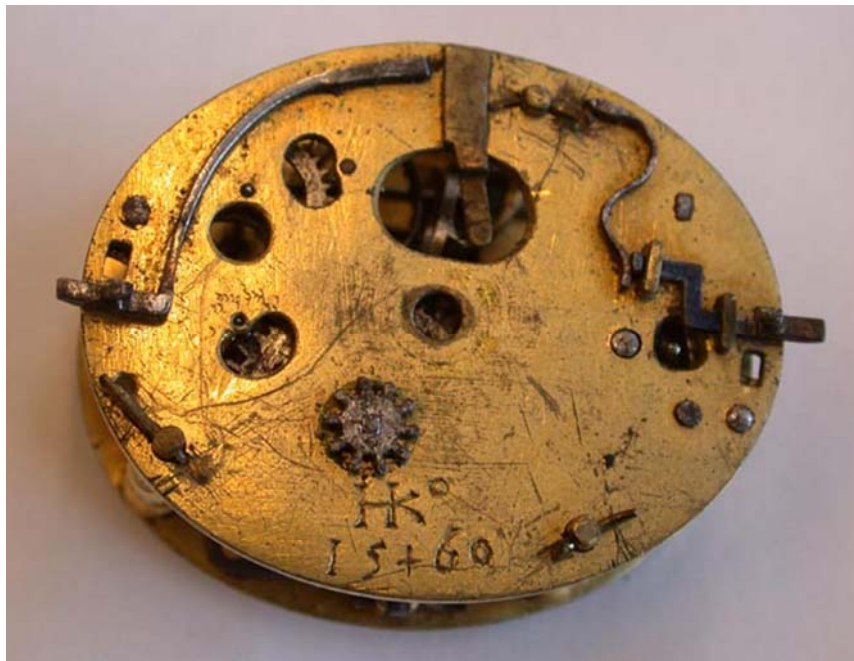
Figure 8. Dial plate, located under the dial of watch (WAM 58.31), engraved with initials and date "HK 15+60".
