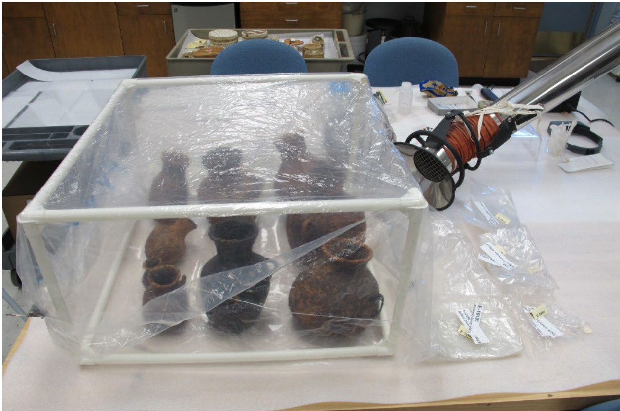
Fig. 7. Solvent chamber for conditioning pitch surfaces (Courtesy of Marilen Pool)
