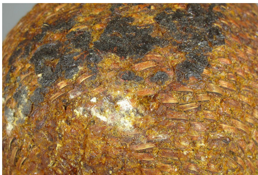
Fig. 3. Lighter-colored pitch exhibiting discolored, crumbling, and brittle surfaces due to oxidation (Courtesy of Marilen Pool)
