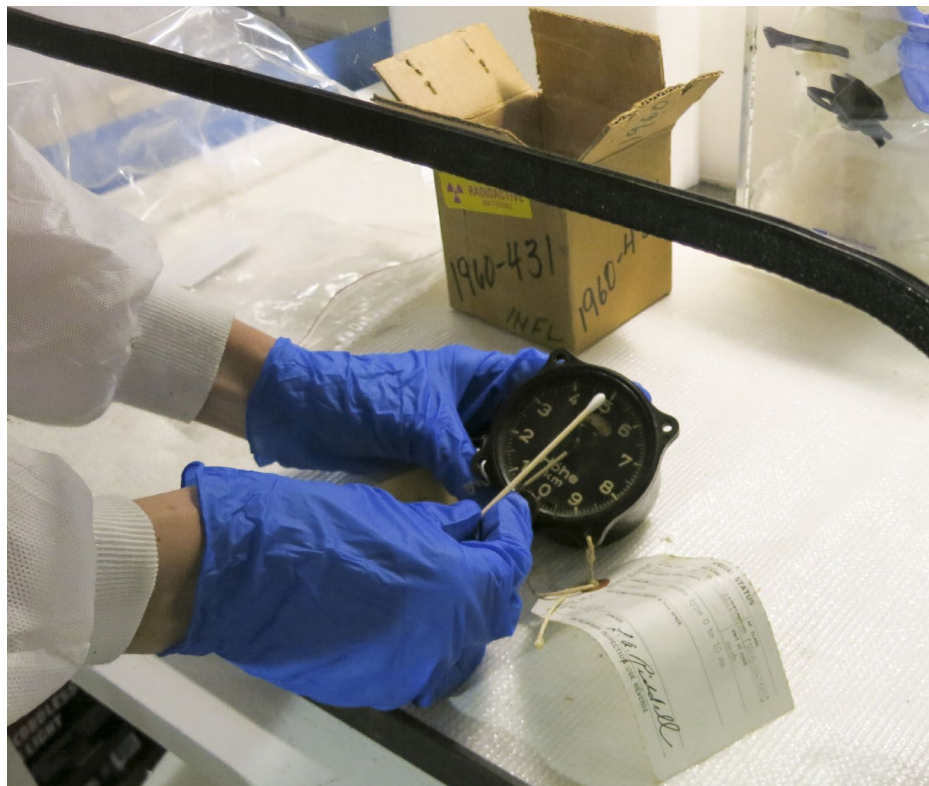
Fig. 2. Taking a wipe from the exterior surface of an instrument face (Courtesy of Amelia Kile)
