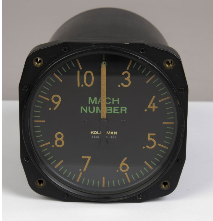
Fig. 1. This Mach meter is an instrument in the display case that contains radium paint. NASM, A19490053000. (Courtesy of Sharon Norquest)
