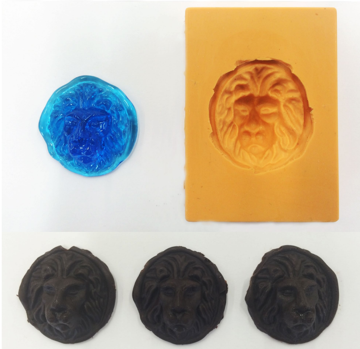
Fig. 1. CopyFlex is a food grade silicone rubber that can be used as a mold for different food items, such as the chocolates pictured here. The authors used the silicone rubber to mold a modern glass lion head to make a dark chocolate version of the glass plaque. (Courtesy of Vanessa Muros)
