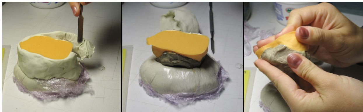
Fig. 8. After curing, the modeling clay walls were peeled away to reveal the cured CopyFlex, which was then easily removed from the figurine mold. (Courtesy of the Ancient Methone Archaeological Project)
