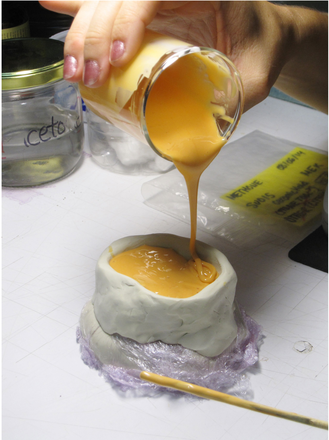
Fig. 7. Pouring the silicone rubber (Courtesy of the Ancient Methone Archaeological Project)
