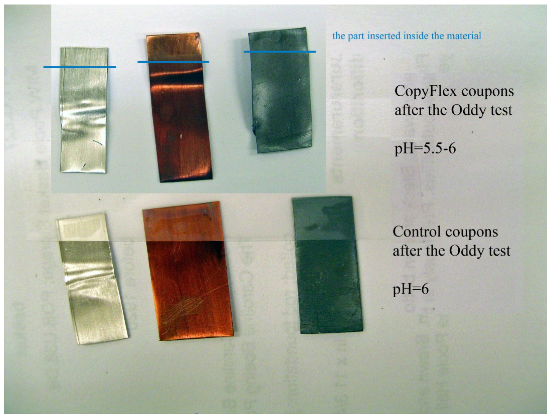
Fig. 13. Results of Oddy test 1 showing the test coupons and the control (Courtesy of Özge Gençay Üstün)
