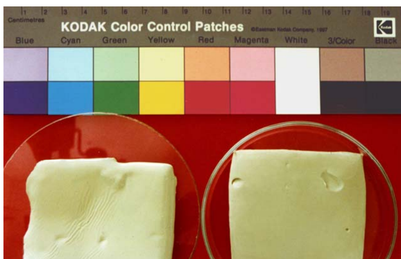
Figure 5. Left, Groomstick exposed to 28 days of natural sunlight; right, Groomstick control.
