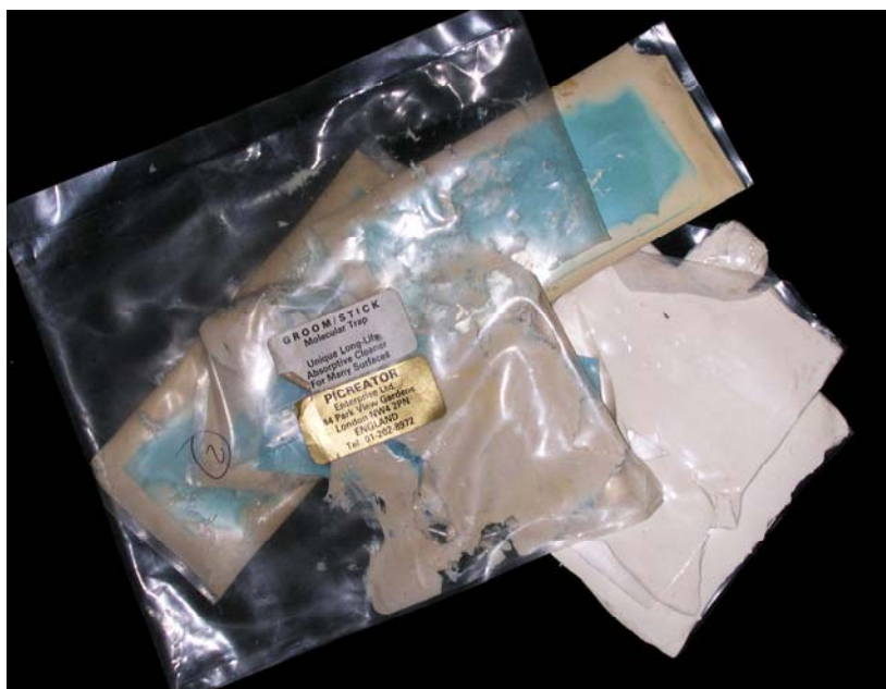
Figure 2. Groomstick samples of unknown age showing typical signs of oxidation.
