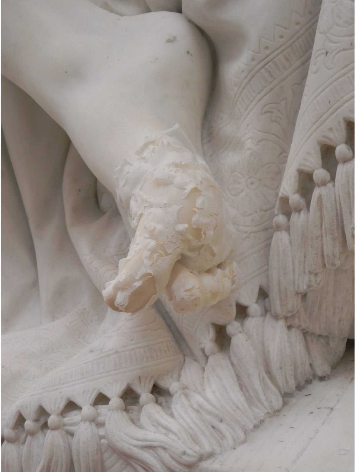
Fig. 6. Dried methyl cellulose poultice on the foot of La Première Pose illustrating film disruption from addition of a chelator (Courtesy of Philadelphia Museum of Art, photograph by Raina Chao)
