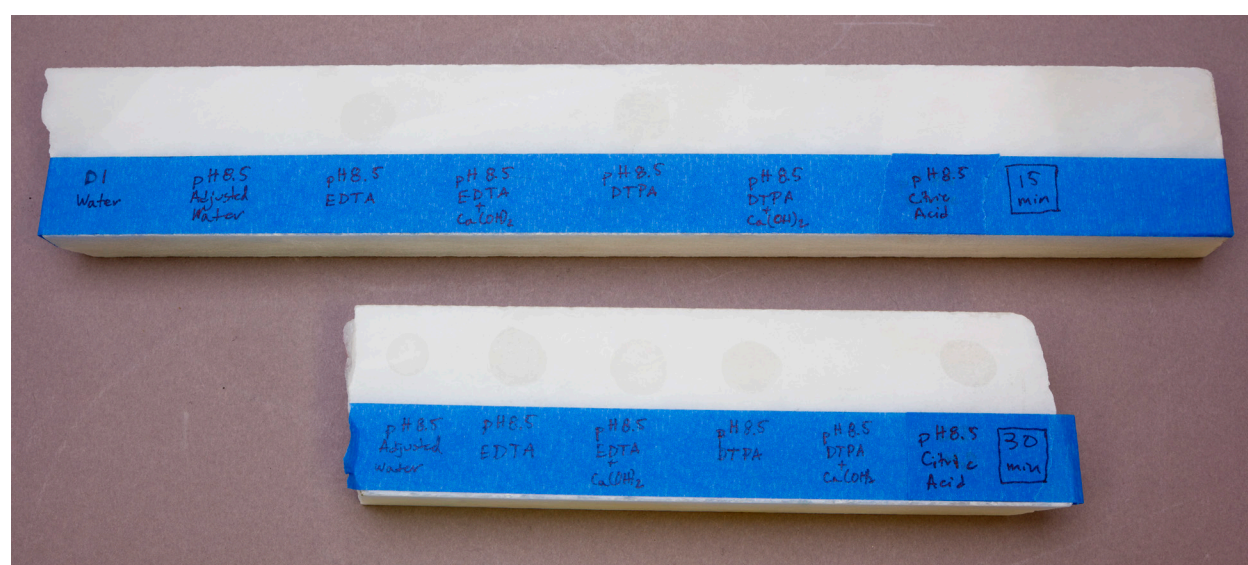
Fig. 17. Test results showing effects on a polished marble surface by buffered pH 8.5 chelating solutions with and without added calcium hydroxide at dwell times of 15 and 30 minutes
