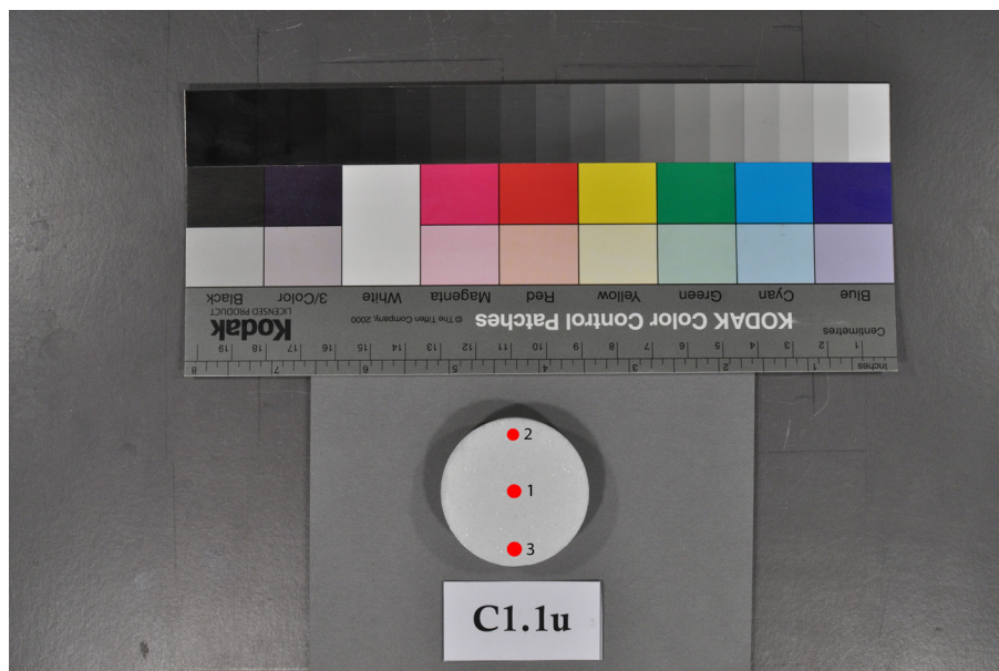
Fig. 5. Marble sample with red dots indicating the points where colorimetry data were collected
