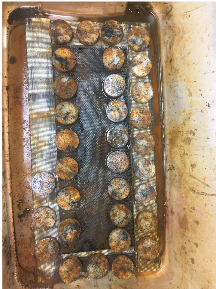
Fig. 3. The marble samples during the staining process
