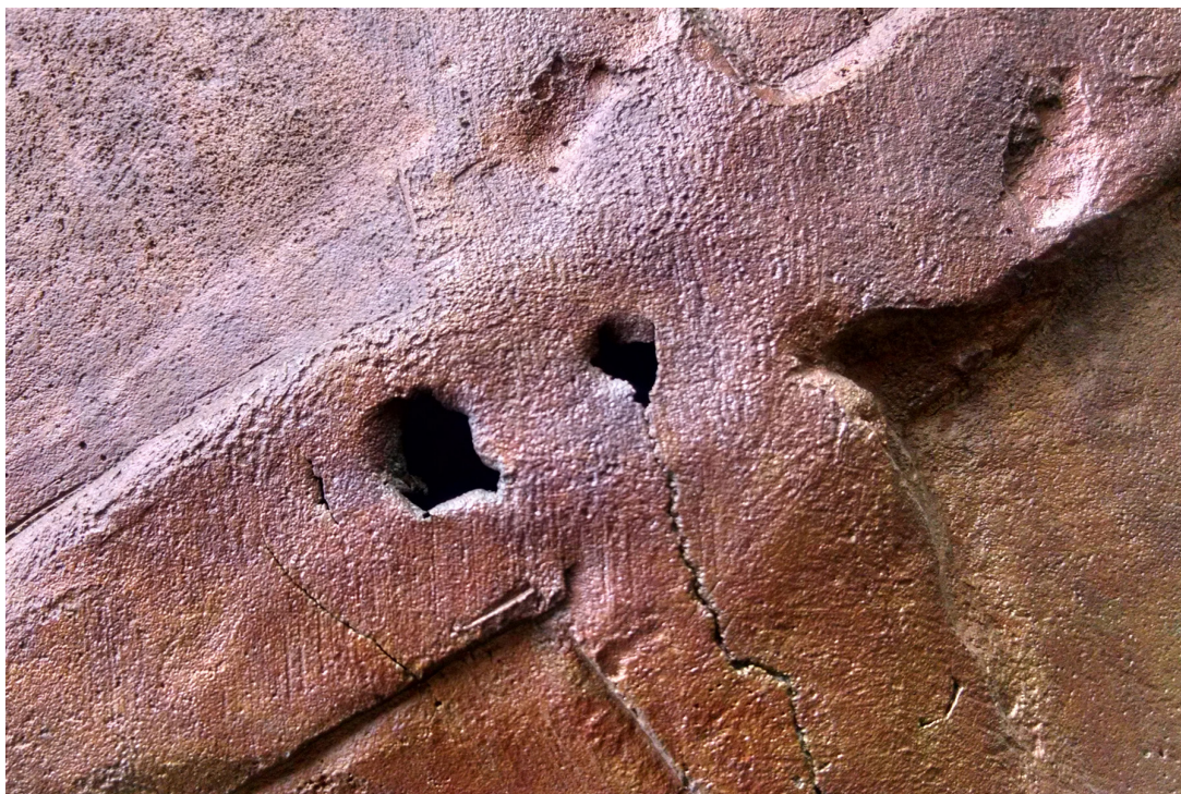
Fig. 15. Detail of voids in King Jagiello cast
