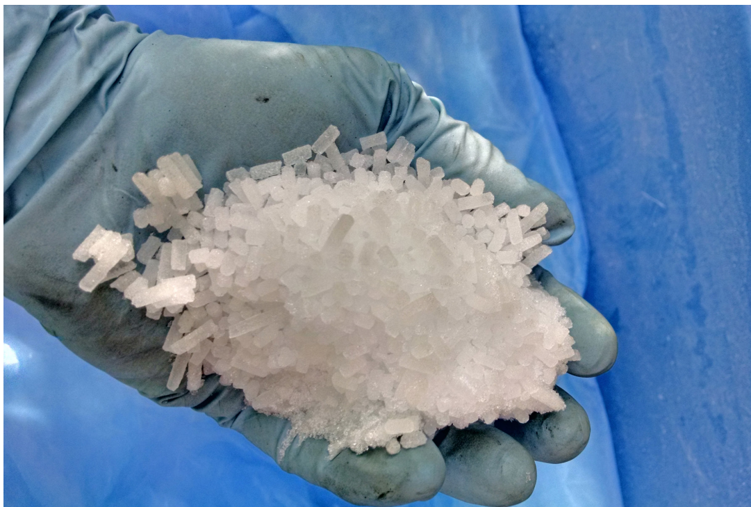
Fig. 6. Photograph of 3-mm diameter dry ice pellet media
