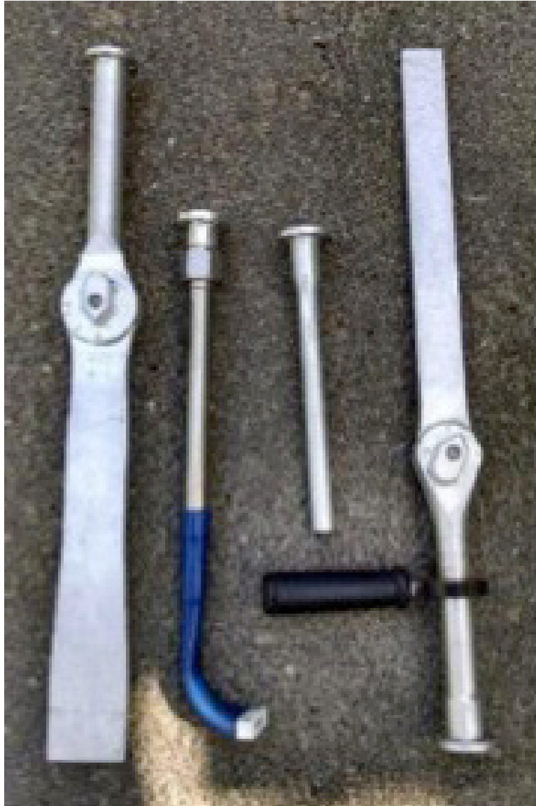
Fig. 11. Assortment of dry ice blasting nozzles with MERN-type #323v1 and #323v2 at the outer edges and the shorter conical nozzle #310S.5 at center right
