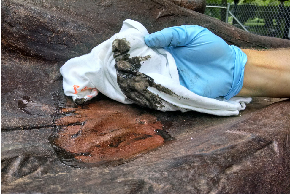
Fig. 8. Gel stripping test confirming that brown coloration was a pigmented coating
