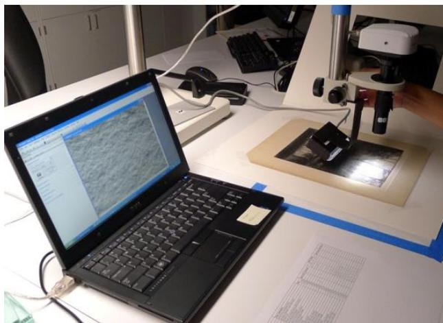
Fig. 4. Micro-Raking Documentation with Texturescope
