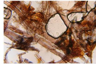
4. All fibers stained red with Graff C-stain. Note short fragmented fibers. Black line is an air bubble.
