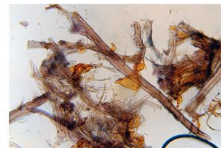
3. All fibers stained red with Graff C-stain. The yellow-stained articles are protein-based adhesive.
