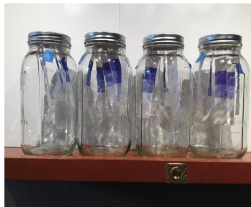
Fig. 3. Diazotype samples are suspended in glass jars with glycerol mixtures to control environmental conditions.
