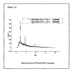
The EDX spectra show a marked amount of platinum is present ON the particle and OFF the particle. This lead to the examination of the amount of platinum present OFF the particle on randomly selected tone 10 samples compared to a tone 00 of a sample (a sample with no platinum). The resulting EDX of OFF particle locations of the Aged Un-washed, Aged Washed 180 min., Un-aged Un-washed tone 10 samples is pictured in *figure 15*.
