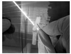
**Figure 10.** Tacking shard in place with sticky wax.
