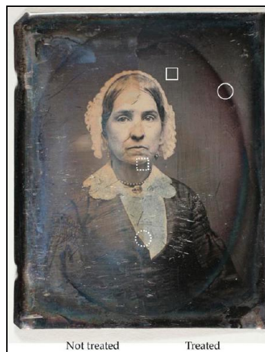
Figure 2. The four areas examined with the usurf confocal microscope. The solid white square (Area A, \square ) is on a grey mid tone area; the solid white circle (Area B, \circ ) is on a portion of the dark blue tarnish oval; the broken line white square (Area C, broken \square ) is on the chin-neck area; and the broken circle (Area D, broken \circ ) is on the jacket-shirt area. The broken square and broken circle show not-treated and treated transition areas.
