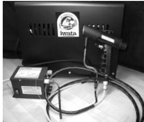
Fig. 7. Anti-static ionizing gun (190 HP from Electrostatics ) attached to air compressor
