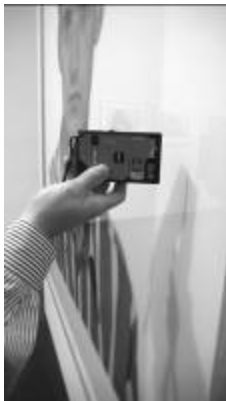
Fig. 6. Measuring static on face-mounted photograph
