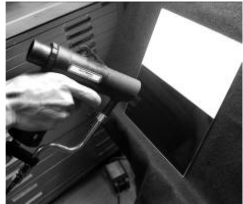
Fig. 8. Using the anti-static ionizing gun to clean a face-mounted sample
