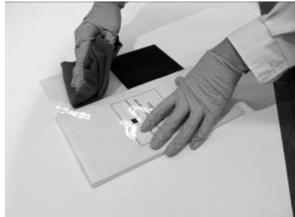
Fig. 4. Left side of sample is covered while right side is cleaned with the various systems
