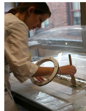
Figure 11. Coating photograph through access portals of humidification dome.
