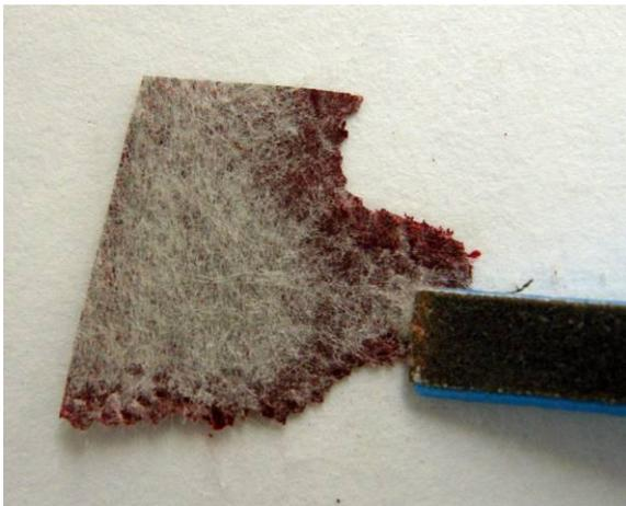
Fig. 8. The verso of a cast composite fill is sanded to expose the cast film along the edge.
