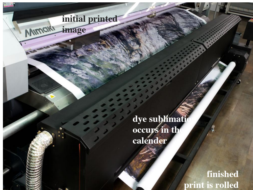
Fig. 12. Thermal energy causing the ink sublimation in textile printing.
