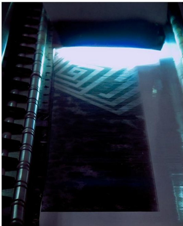
Fig.11. UV radiation causing the photopolymerization of direct printing inks: the UV light source is passing over the applied ink, causing it to cure.
