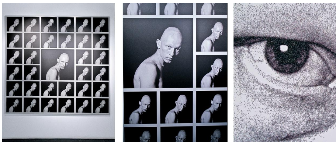
Fig. 15. A direct printed image on a Dibond support, overall ( left ) and detail images ( center and right ). The digital halftone screen patterns produced by the inkjet printer are visible upon close examination.
