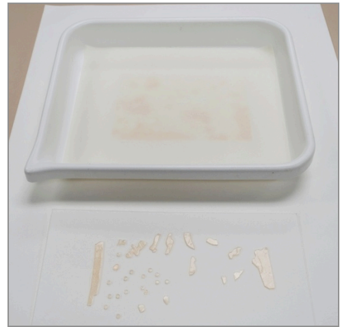
Fig. 15. Pink discoloration in gels and blotter indicate successful iron chelation in treated areas
