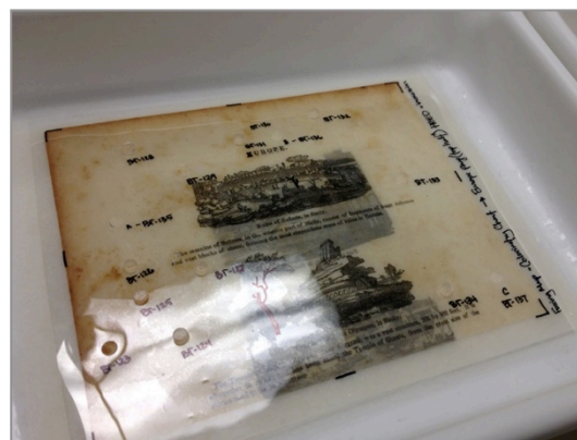
Fig. 8. Template used to facilitate gel placement and instrument registration.
