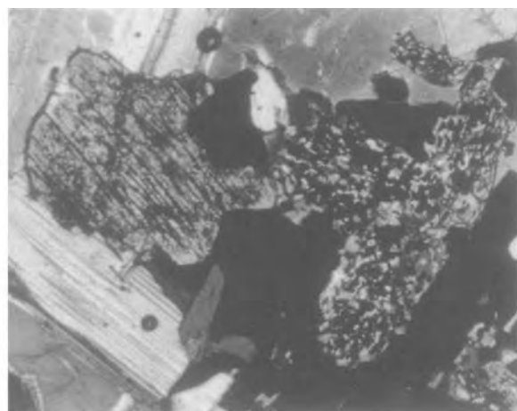
Figure 7, 50x, transmitted light w/crossed polars, silicates filled with magnetite and ilmenite euhedra
