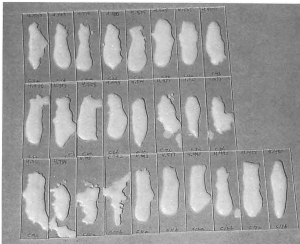
Figure 1. Cyclododecane applied by pipette in the melt on glass microscope slides.
