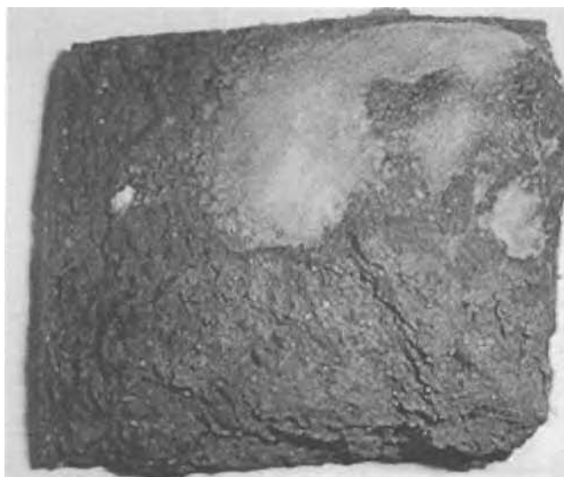
Figure 8. Test Brick #4, after six months, cyclododecane partly sublimed.
