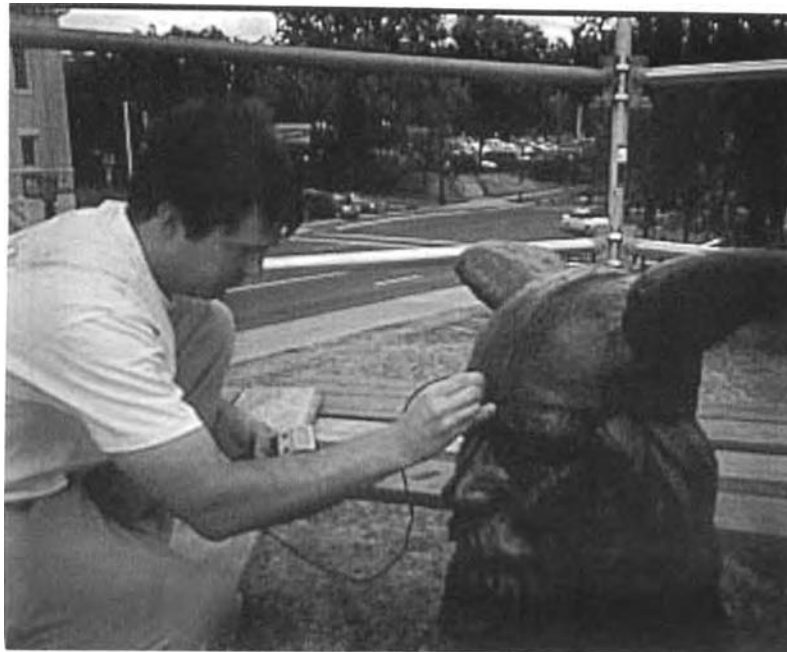
Figure 14. CTA staff taking coating thickness measurements on the head of Leif Erickson after treatment, 1996.
