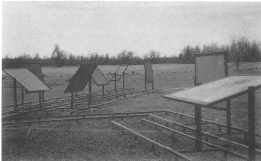
Figure 14. Formula Compound #1 . The banks of panels showing corrosion, paint loss and missing pieces. March 2002
