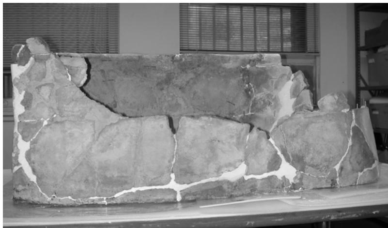
Figure 9. Coffin during reconstruction showing breaks along the horizontal center seam (square back end is to the left, rounded end to the right).
