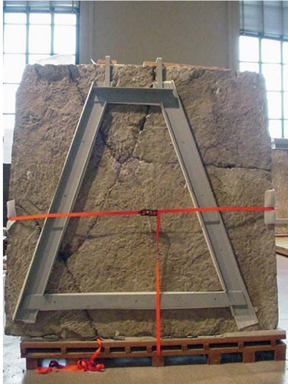
Figure 16. Backing in place with hanging hooks at top.
