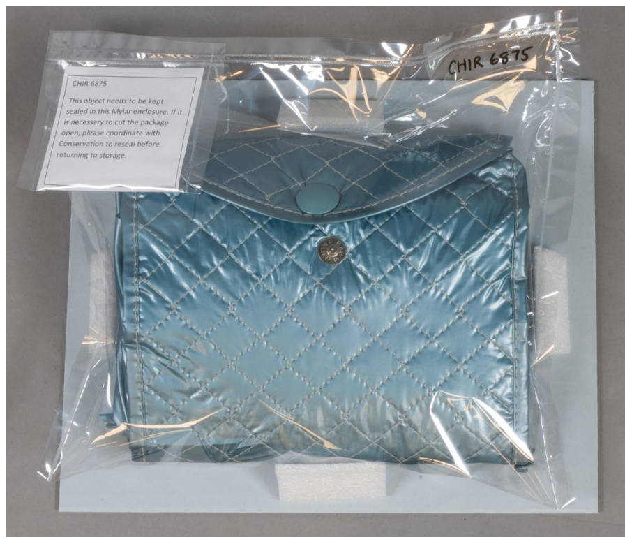
Fig. 13. Plasticized PVC object enclosed in sealed Mylar and set on a handling tray. National Park Service, Chiricahua National Monument, CHIR 6875 (Courtesy of Maggie Hill-Kipling)
