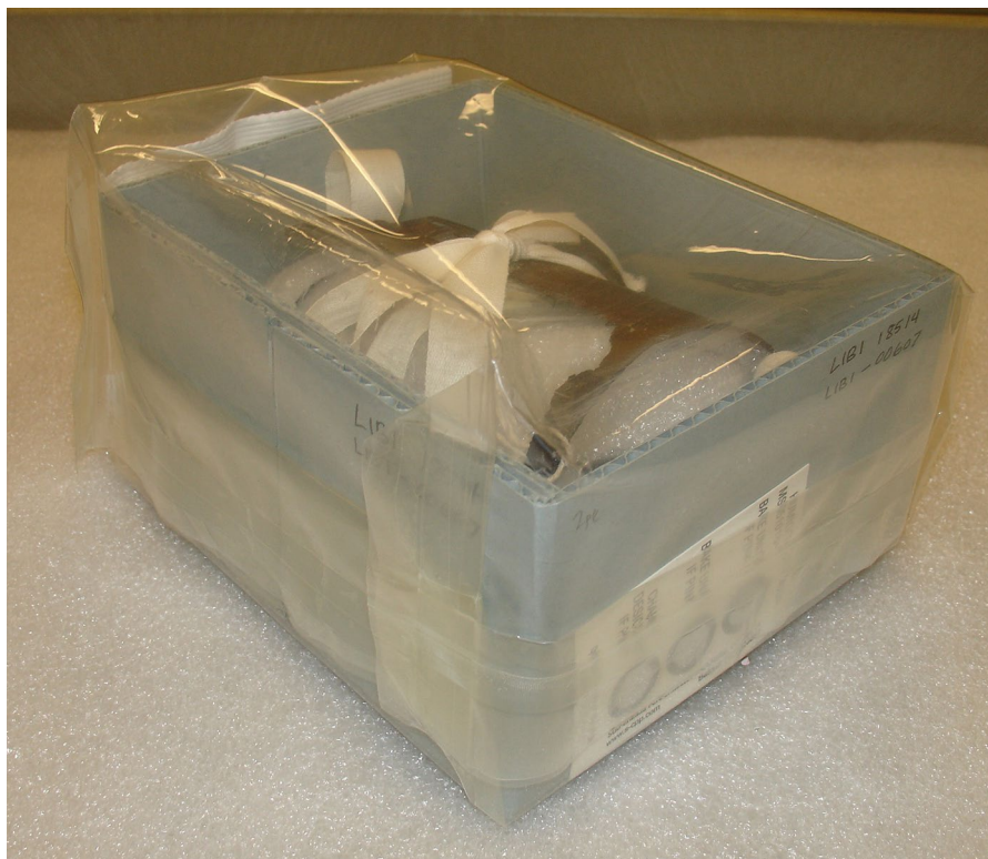
Fig. 1. Example of an object in tray enclosed in Escal vapor barrier bag (Courtesy of Dana K. Senge)
