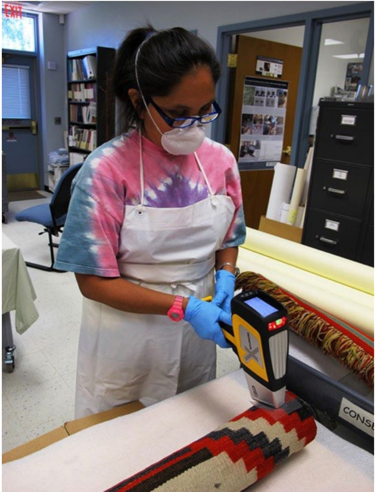
Fig. 3. Personal protective equipment worn while conducting pXRF testing on textiles (Courtesy of Gina Watkinson)
