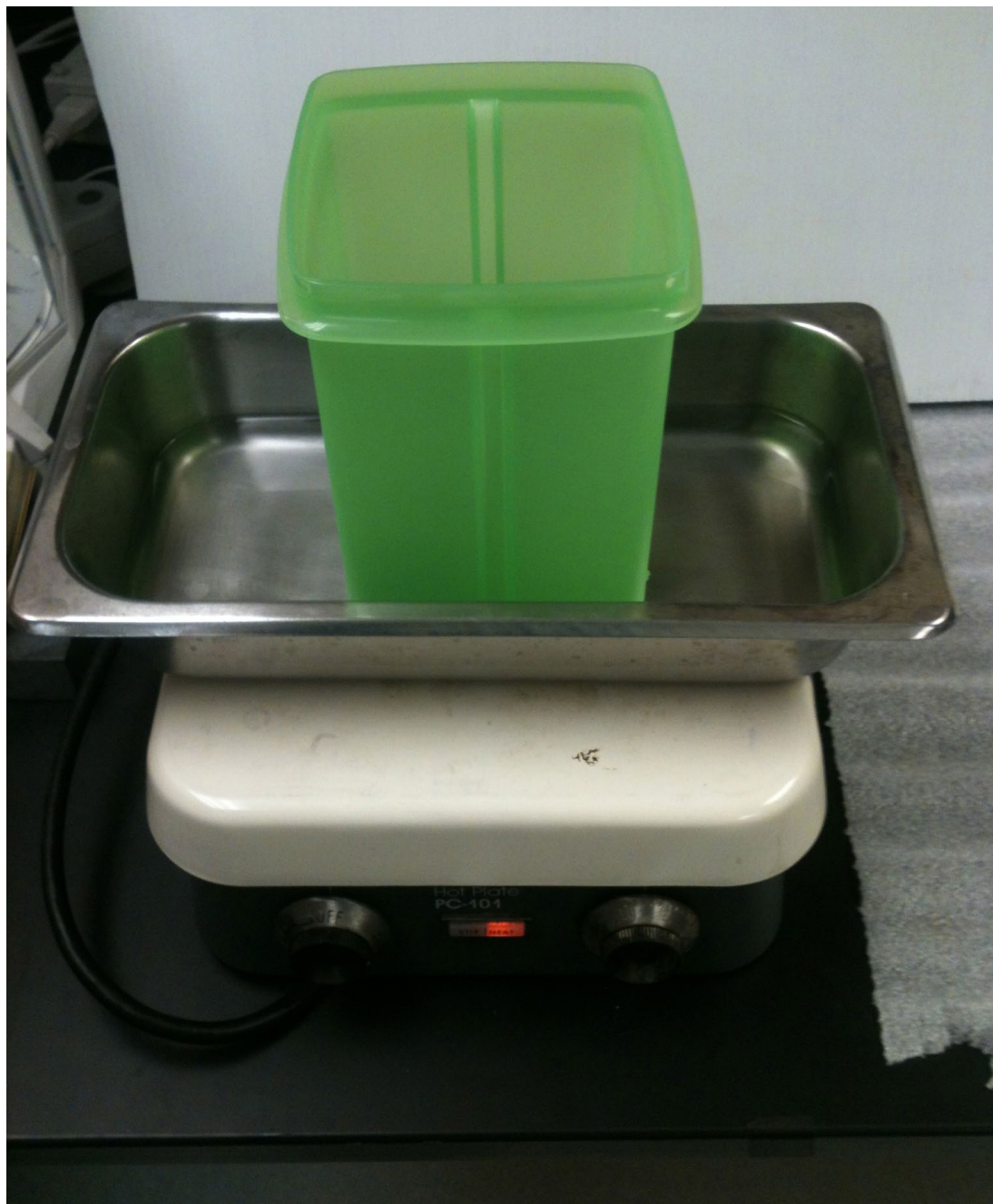
Fig. 11. Temperature test setup (Courtesy of Jae R. Anderson)
