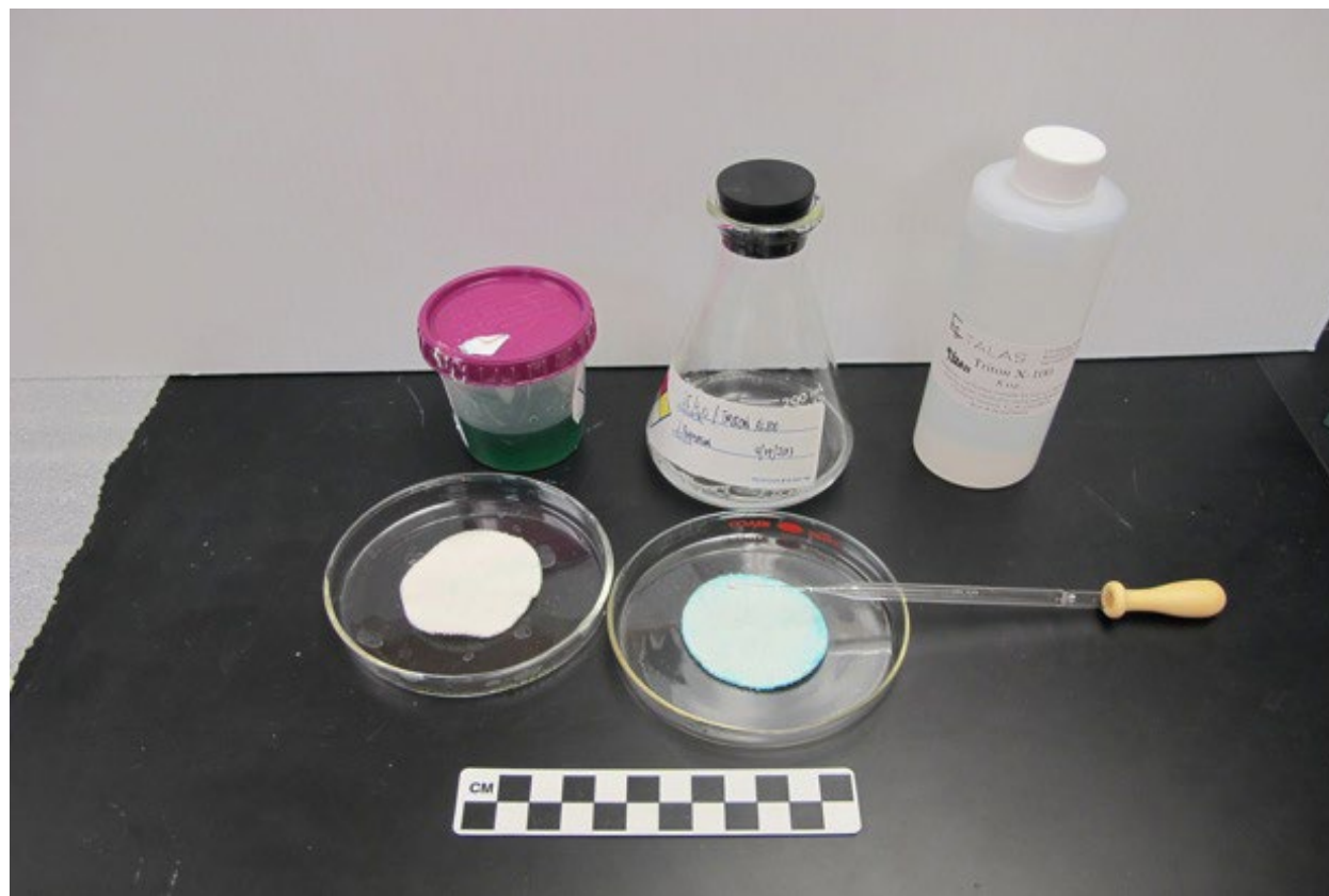
Fig. 6. Homogeneous absorption into cotton sample: deionized water, Triton X-100, and McCormack food coloring (Courtesy of Jae R. Anderson)
