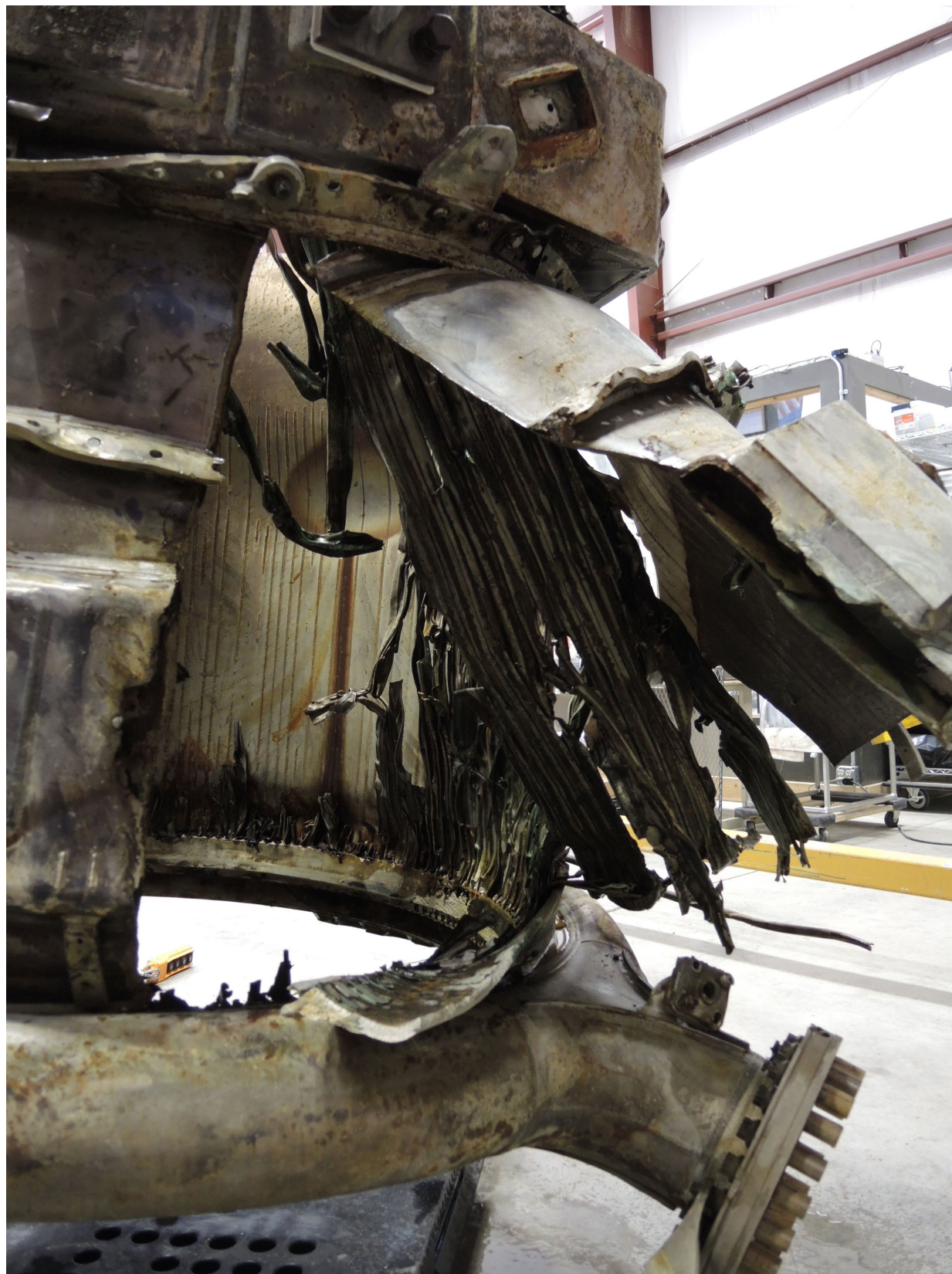
Fig. 6. Ruptured jacket from a thrust chamber belonging to engine #5 from Apollo 11 (Courtesy of Terra Mare Conservation LLC)
