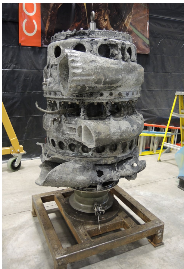
Fig. 12a. Turbopump F1-2013-0045 after conservation (Courtesy Terra Mare Conservation LLC); 12b. Original photo showing a similar turbopump on the assembly line (Courtesy Rocketdyne Harold C. Hall Collection)
