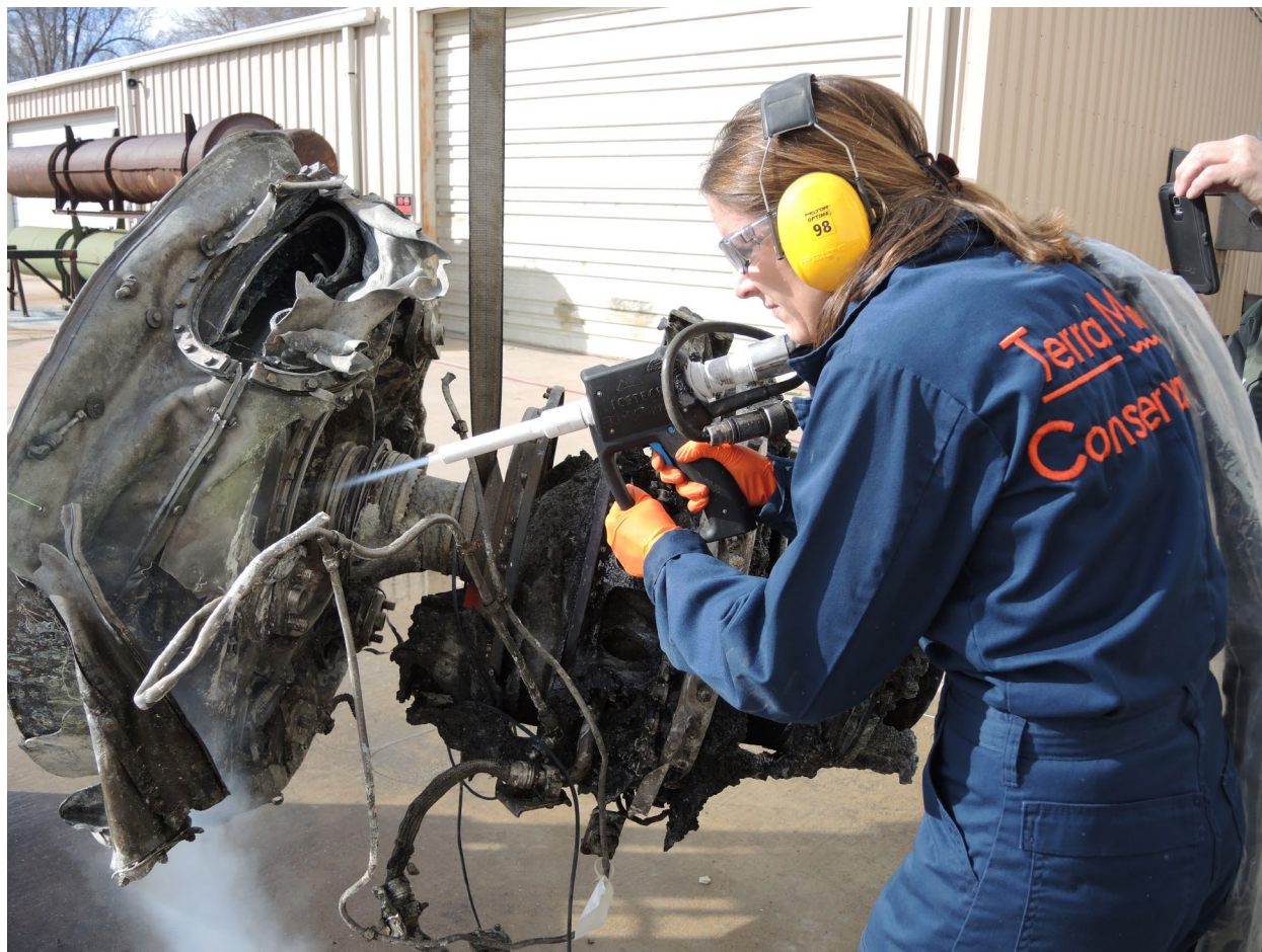
Fig. 14. Conservator Claudia Chemello cleans turbopump F1-2013-0012 with dry ice (Courtesy of Terra Mare Conservation LLC)
