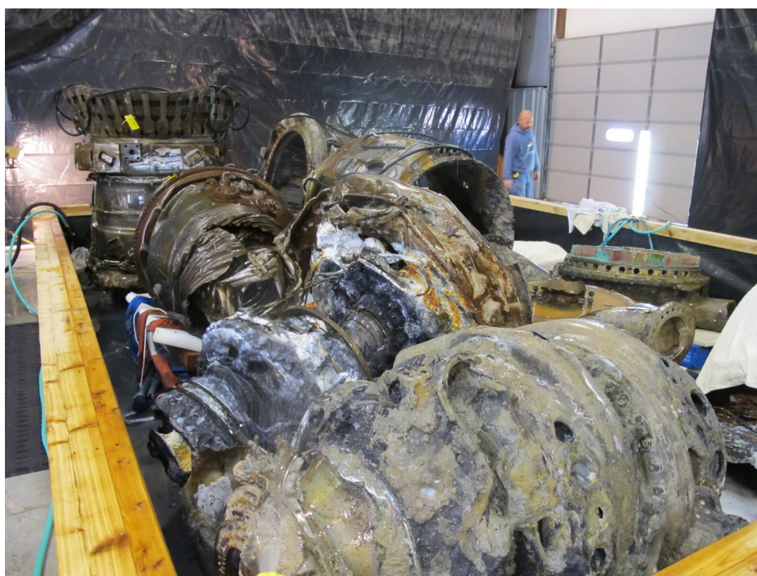
Fig. 3a. View of the lab with recently recovered artifacts in custom-fabricated basins; 3b. Detailed view of basin #1 with turbopumps in the foreground (Courtesy of Terra Mare Conservation LLC)
