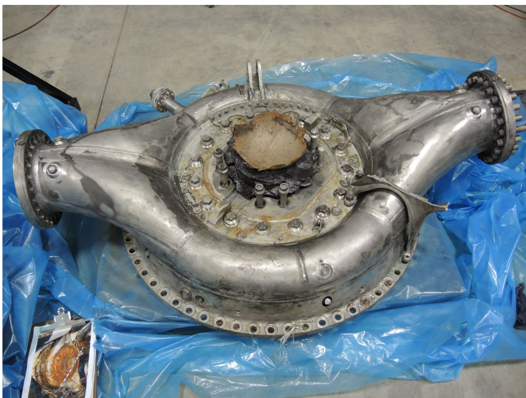
Fig. 10a. Lead Technician Jerrad Alexander (left) and Conservator Paul Mardikian (right) removing the steel gimbal from Apollo 11's LOX dome F1-2013-0005-1 for conservation; 10b. The same LOX dome and gimbal after conservation (Courtesy of Terra Mare Conservation LLC)
