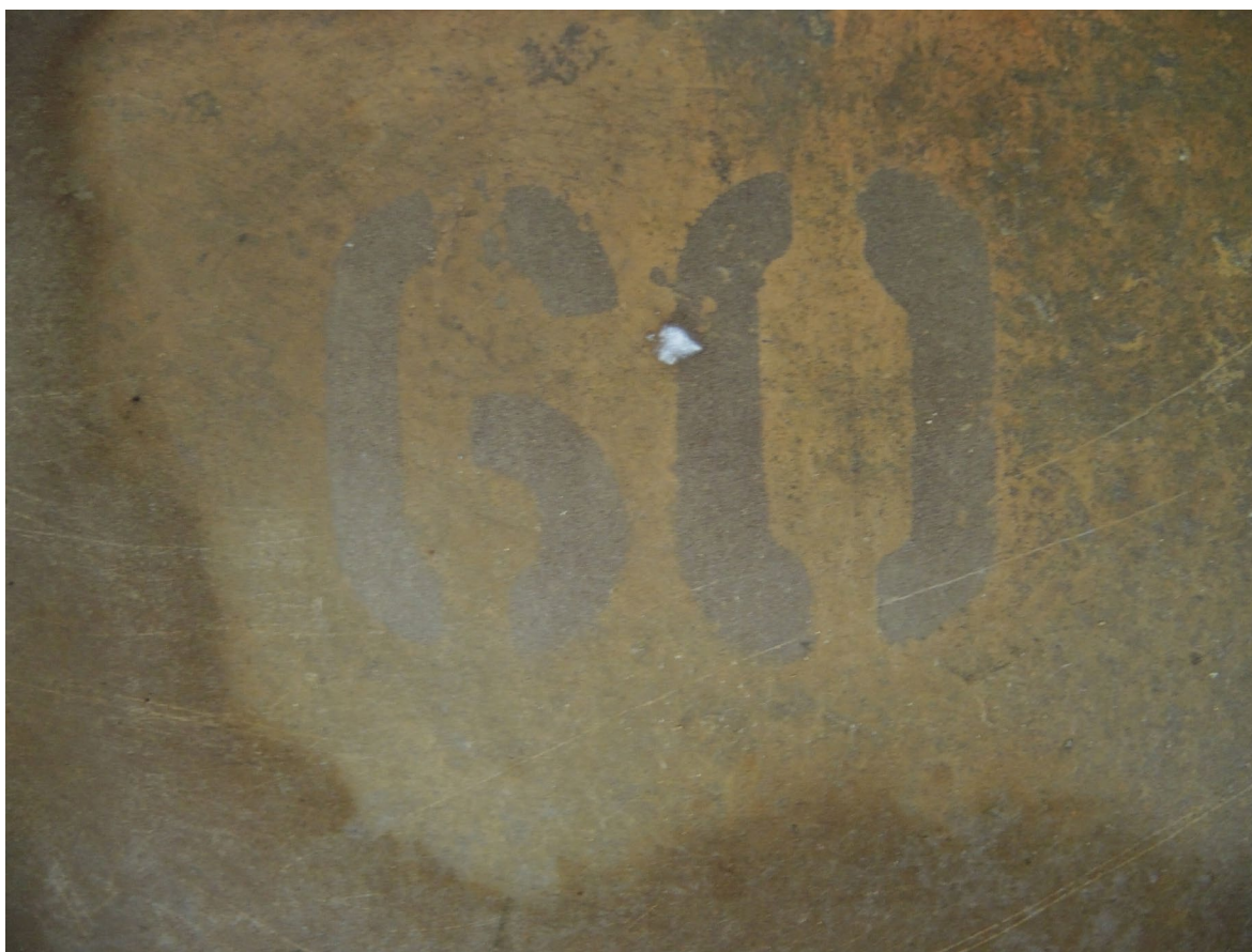
Fig. 4a. Example of a stenciled number on a thrust chamber only visible due to the presence of rust surrounding the numbers (Courtesy of Terra Mare Conservation LLC)
