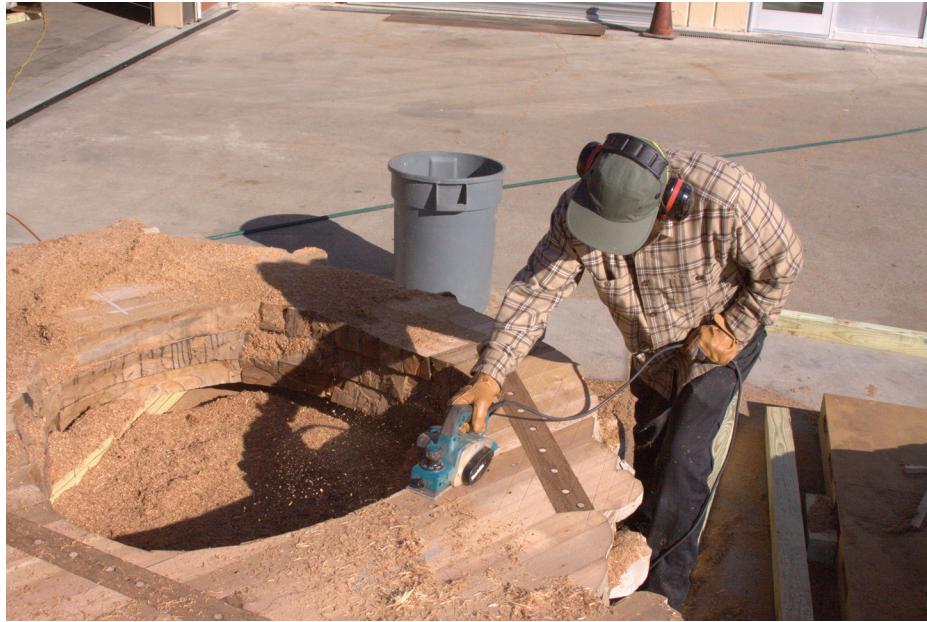
Fig. 8. Planing of a section to the determined measurements (Courtesy of Ursula von Rydingsvard, photograph by James Gouldthorpe)
