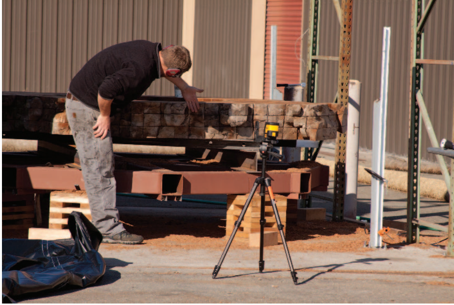
Fig. 6. Sean Weeks-Earp identifies high and low points in a section using a laser level and customized setup (Courtesy of Ursula von Rydingsvard, photograph by James Gouldthorpe)
