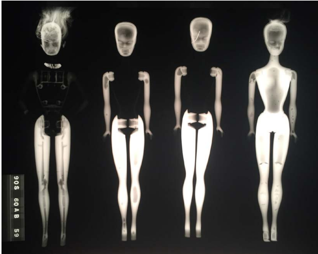
Figure 4: X-Radiography image of the c.1959 doll (far right). For comparative purposes, two dolls from the 1960s (middle), and one doll from the 1990s (far left) were also examined. X-rays collected at 35 kV, current of 6.85 \mu A for 120 seconds with a focal distance of 1 meter and a focal spot of 2.5 mm.
