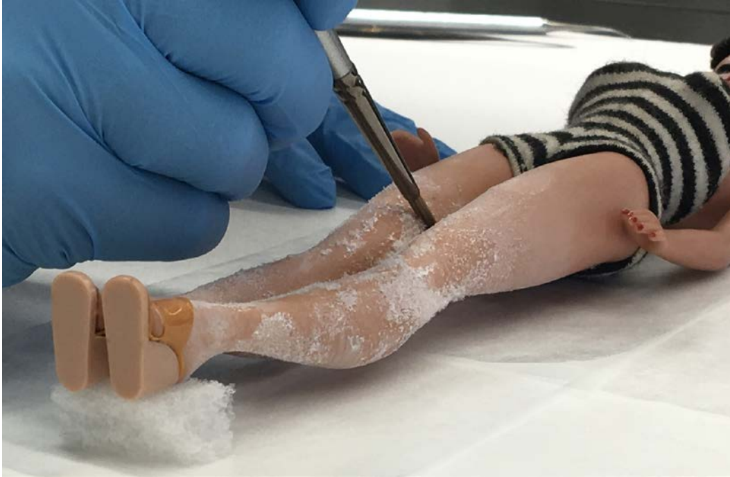
Figure 8: Mechanical removal of the white efflorescence from the c. 1959 Barbie legs with a soft brush. The exudate was collected and stored in plastic vials for future study.
