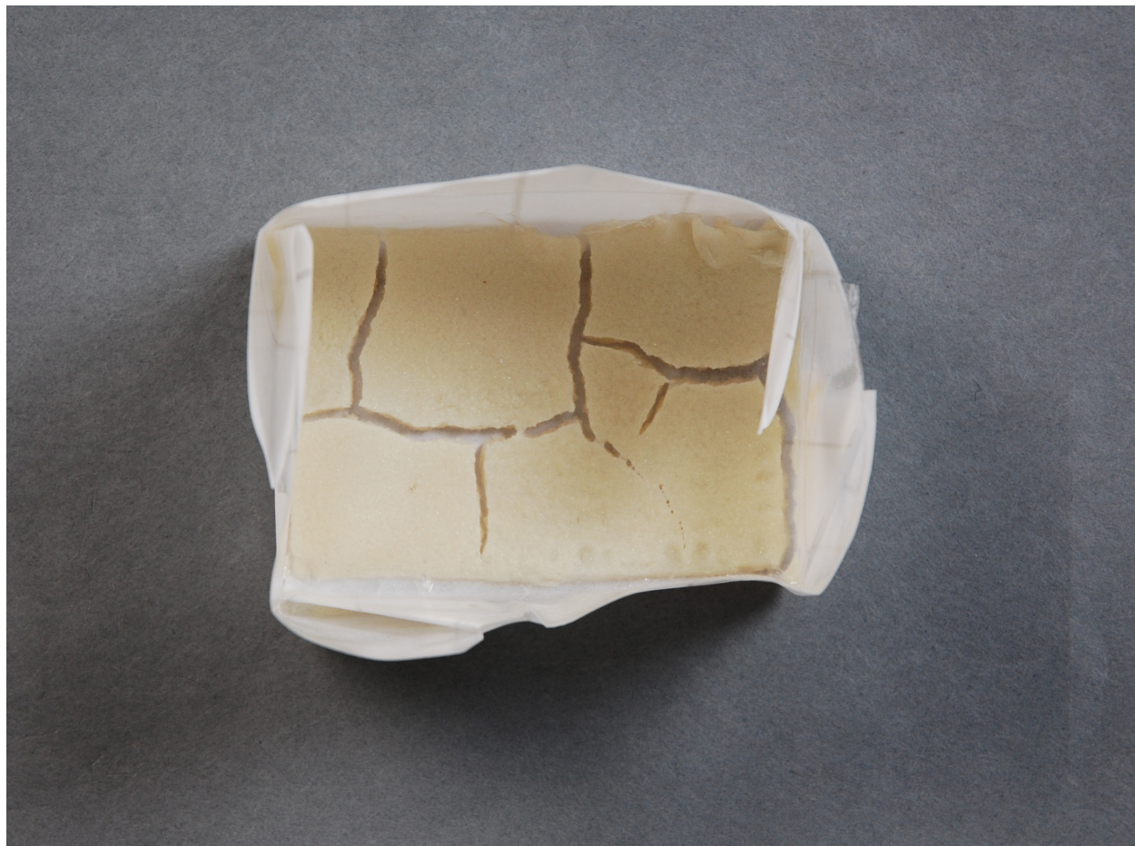
Fig. 4. Cracking caused by the addition of too much dry pigment, resulting in oversaturation and loss of cohesive strength
