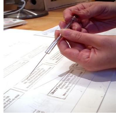
Fig.10. Applying solvent by micropipette.
