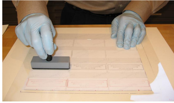
Fig.5. Applying stamps through a polyester template onto the samples lying face-down on matboard.
