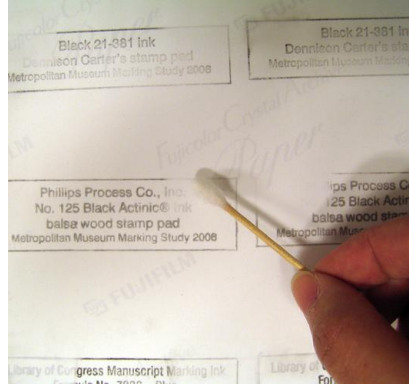
Fig.9. Applying solvent with a cotton swab.
