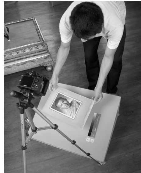
Fig. 5. The simple stage setup for digital photography of oversized prints.
