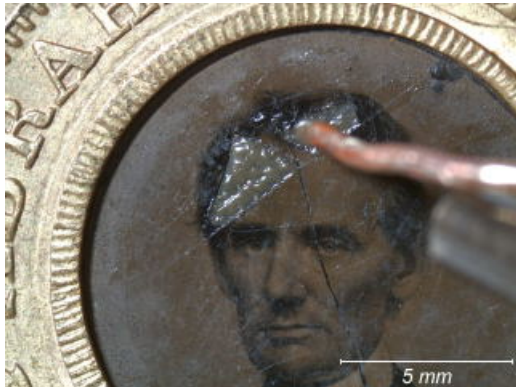
Fig. 6. Application of wax-resin mixture. 6.5X
