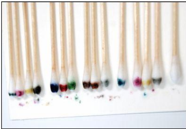
Figure 3 Cotton Swabs Used to Clean Ilford 3 with Ethanol and Water
