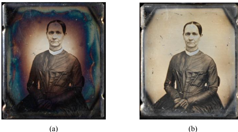
Fig. 8 - Visual comparison of a daguerreotype a) before and b) after electrochemical cleaning at -1.3 V (ESS).
