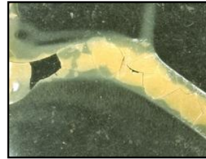
Figure 4b. Detail of cracking varnish on collodion wet plate negative. 6.25x magnification. Courtesy GRI.
