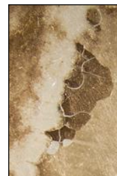
Figure 8b. Detail of cracking collodion emulsion on a wet plate negative. 6.25x magnification. Courtesy GRI.
