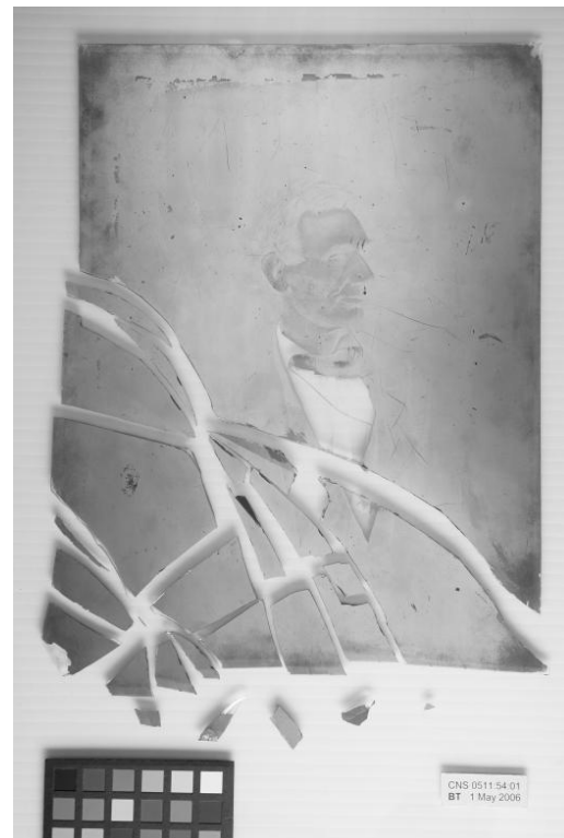
Fig. 3. Silver mirroring visible on the surface.
