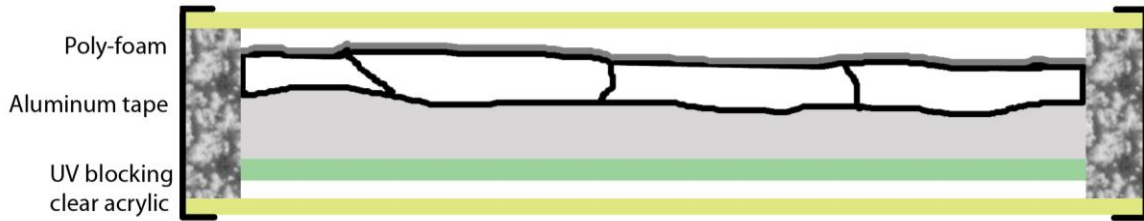
Fig. 5. A cross section of the plate package's housing.
