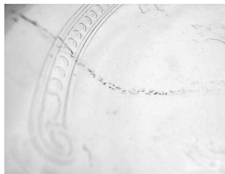
Fig. 4. “Snowflakes” formed within a break mended with Paraloid B-72.
