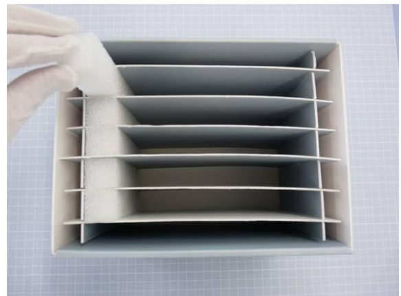
Fig 20. After assembling the partitions, the sides were filled with Ethafoam strips.
