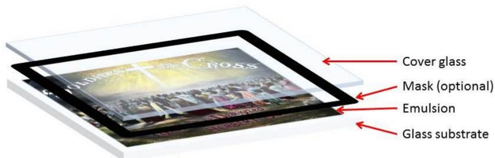
Figure 1: Typical glass slide structure.
