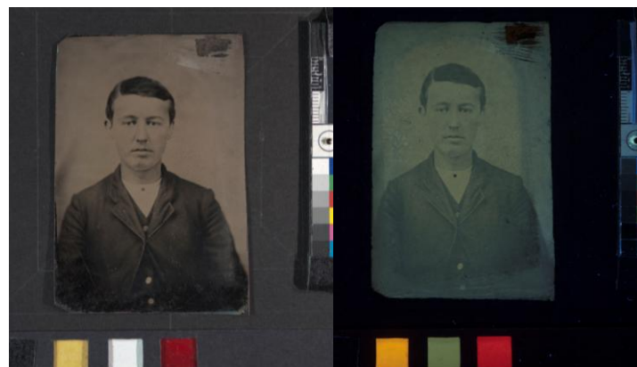
Fig. 7. Normal (left) and UVA-induced visible fluorescence (right) images of a tintype. The image on the right clearly shows how the presence of a paper holder altered production of fluorophores.
