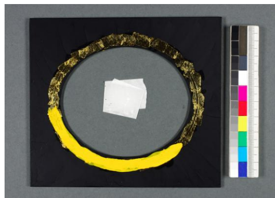
Fig. 28. The gilding is covered with a layer of yellow varnish.
