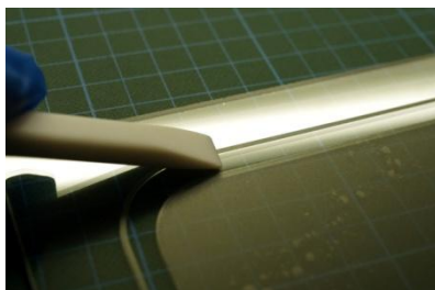
Fig. 17. Applying gentle pressure with a Teflon spatula.
