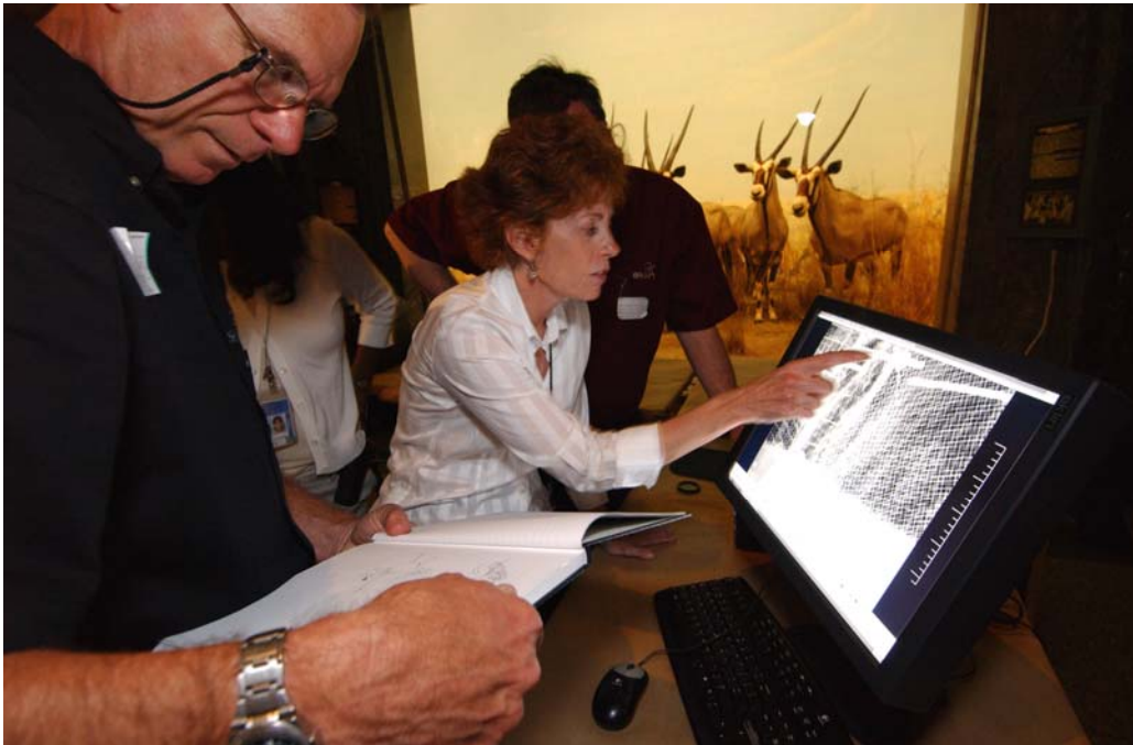
Figure 23. Digital X-radiography in process – x-ray image of internal mounting of ear seen on computer screen.
