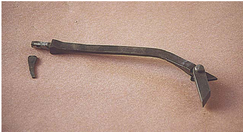
Figure 11. The re-created hour strike release arm.
