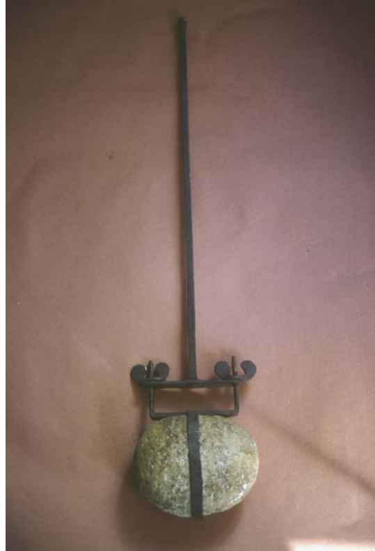
Figure 7. Detail of the weight end of the existing shortened pendulum showing the unique weight stone and wing nut assembly for fine adjustment of pendulum length.
