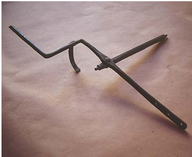
Figure 10. The re-created quarter hour strike lever showing the functional configuration and dimensions of the prototype (Fig. 5).
