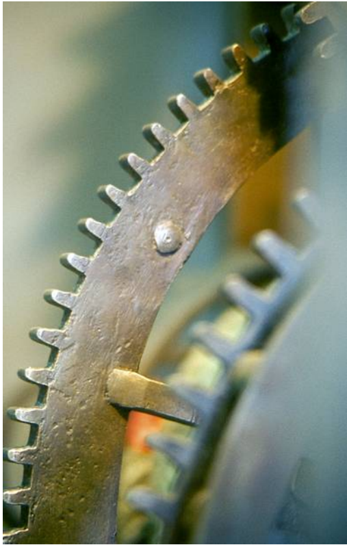
Figure 6. The back of one of four pins on the hour wheel showing a punch mark indicating it as the likely hour lift pin.
