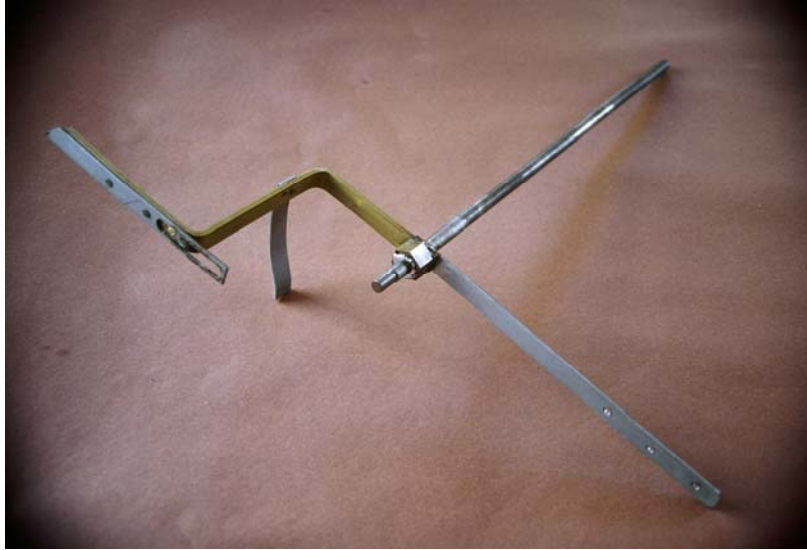
Figure 5. The prototype quarter-hour strike lever.
