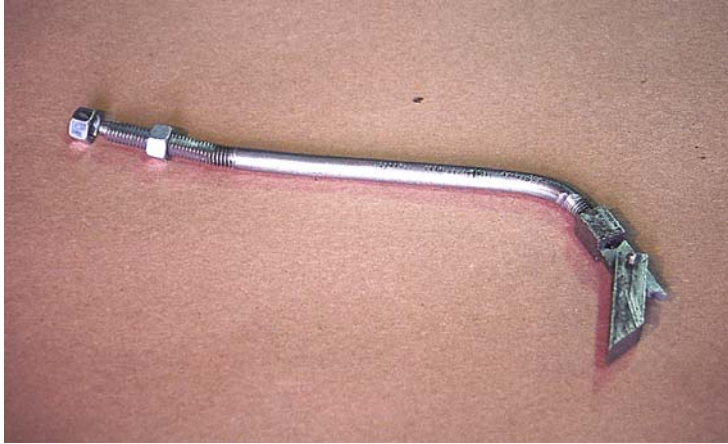
Figure 4. The prototype hour strike release arm.
